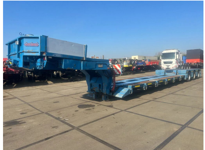
Nooteboom EURO 54-03 3 AXLE STEERING, EXTENDABLE
